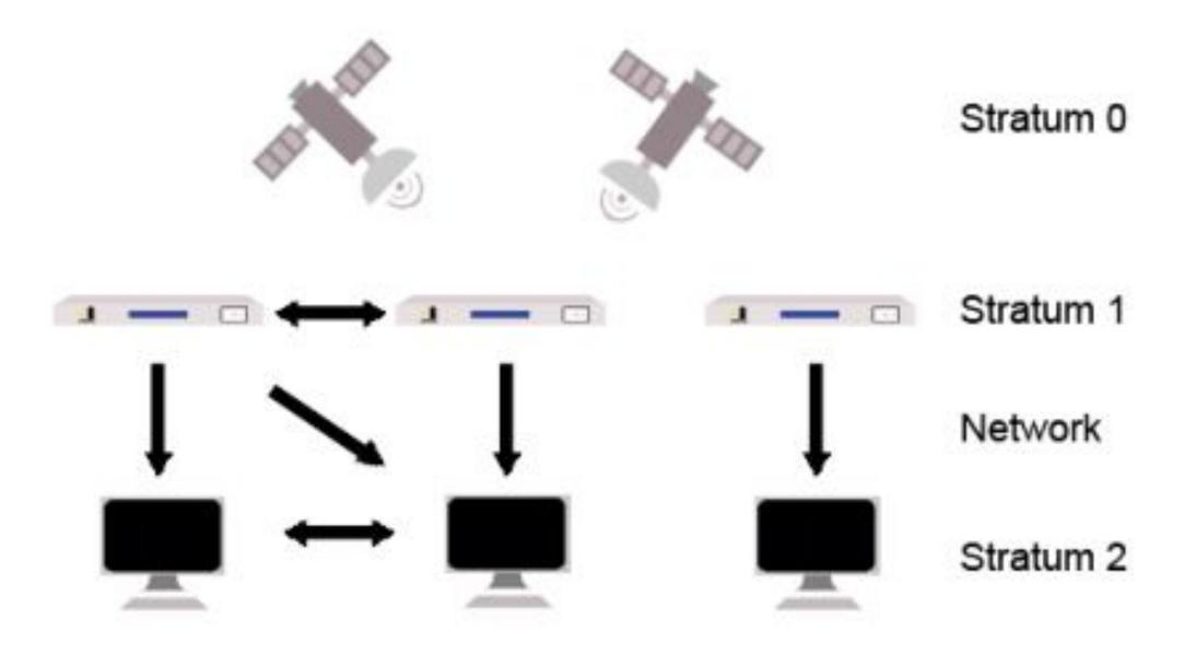
The NTP Stratum model is a representation of the hierarchy of time servers in an NTP network,
